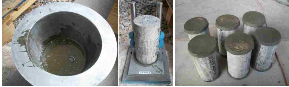
Figure 15. Sulfur capping preparation.
