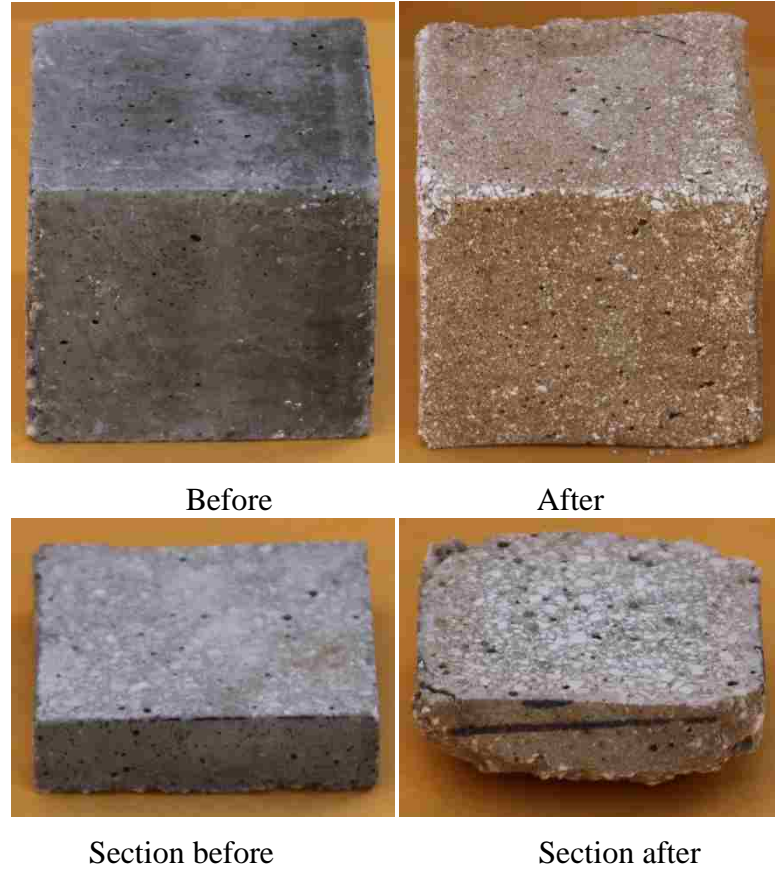
Figure 50. Fly ash based geopolymer before and after the exposure to 800°C.
