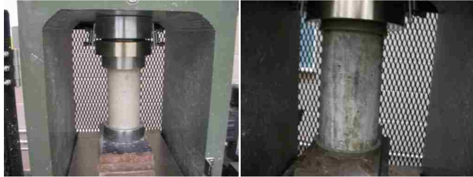
A- Test with unbounded capping
