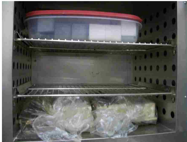
Figure 42. Geopolymer mortars specimens inside an oven.
