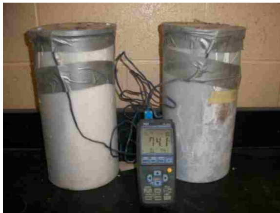
Figure 14. Temperature of freshly mixed concrete test setting.
